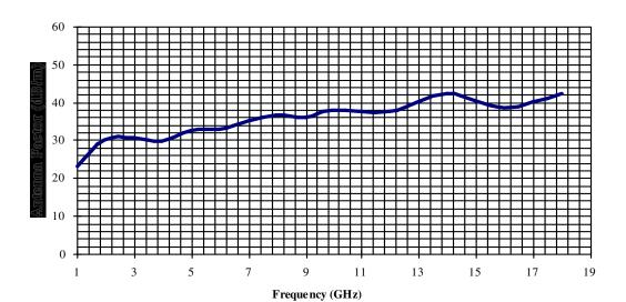
Figure 1-1 Typical Antenna Factors
