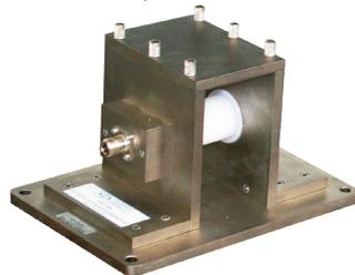
The **FCLC-400** is compliant with the Insertion Loss and VSWR requirements mandated by MIL-STD-461 and RTCA-DO-160.
