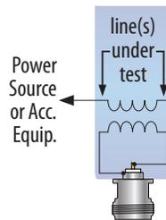
$$\begin{matrix} \text{Measured} \\ \text{Voltage Value} \\ \text{(in dB}\mu\text{V)} \end{matrix} - \begin{matrix} \text{Transfer} \\ \text{Impedance Factor} \\ \text{(in dB}\Omega\text{)} \end{matrix} = \begin{matrix} \text{Current} \\ \text{Value} \\ \text{(in dB}\mu\text{A)} \end{matrix}$$
