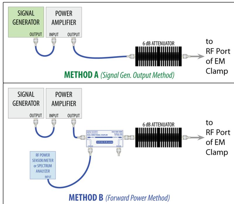
Figure 14 - Examples of Test Generator Equipment
