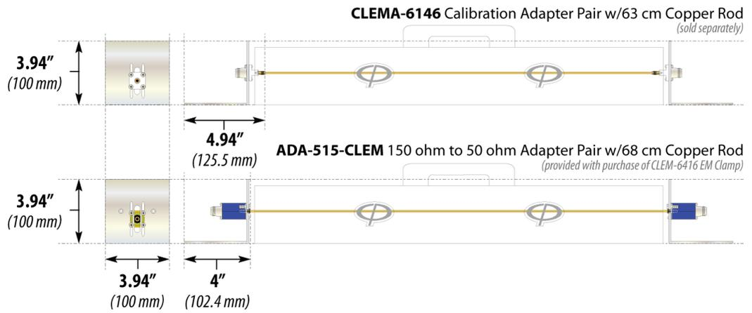
**Figure 4 - Product Dimensions - EM Clamp Adapters and Accessories**
