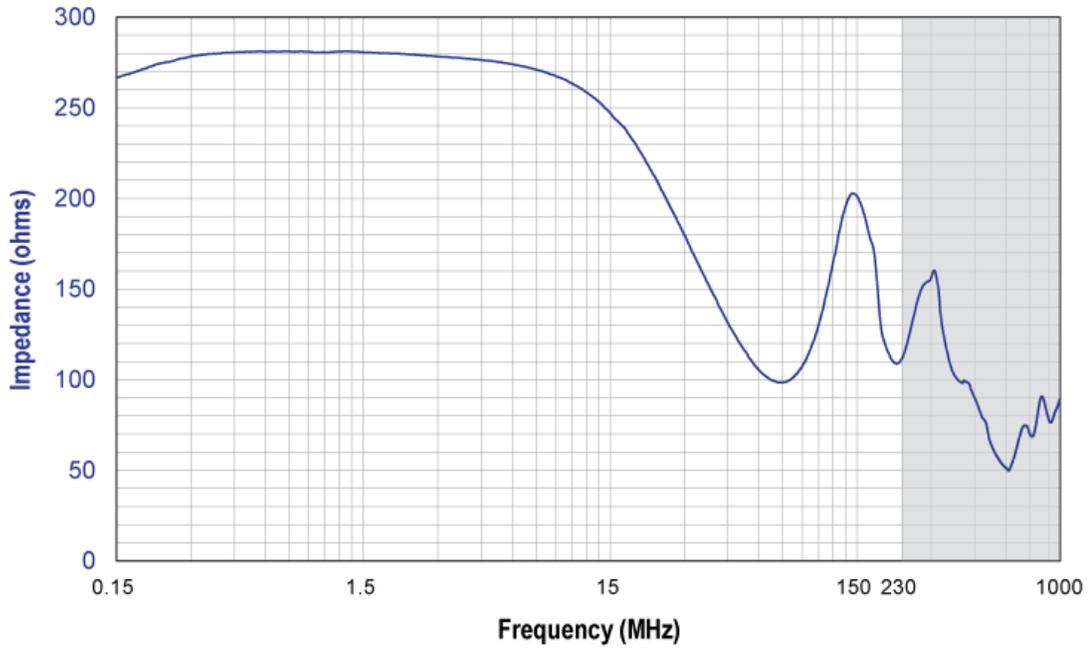
**Figure 7 - Typical Impedance Data**
