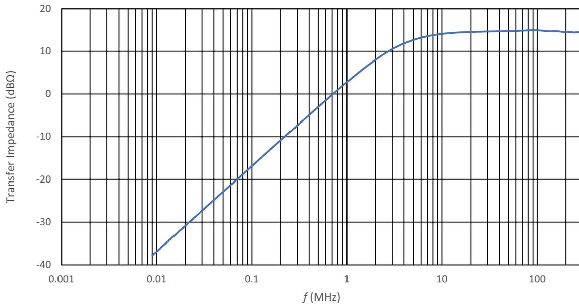
» \* Probe calibrated with 50 $\Omega$  load impedance.
