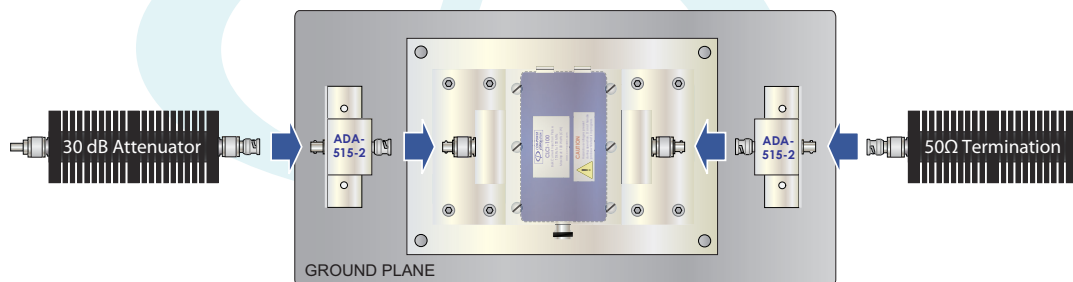
FIGURE 10 - Setup for Calibration Accessories for 150Ω System
