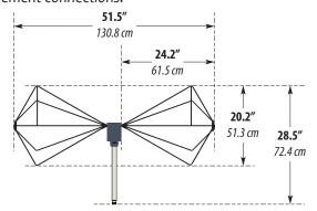
The standard [fixed] antenna elements are constructed using corrosion resistant aluminum which is powder coated for additional durability. Optionally available collapsible elements, constructed from high quality, polished aluminum are also available. The collapsible elements (shown below) expand to the same shape as the fixed elements, with insertable gamme match rods.
