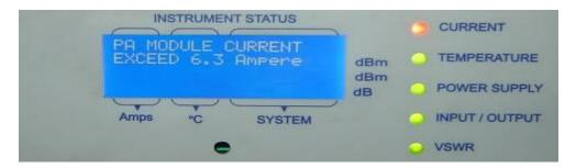
8. In order to restart the unit, first turn off the front panel switch, and then restart the unit as described in Section 3.
