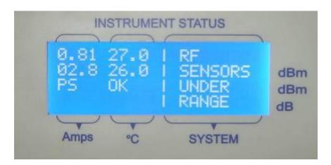
Please note that Pin, Pout, SWR and Gain will not be displayed until the amplifier sees an input of -45dBm.
