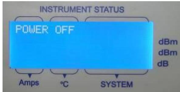
7. Depending on the nature of the fault the appropriate red LED will be light up and the corresponding fault message will be displayed on front panel LCD.
