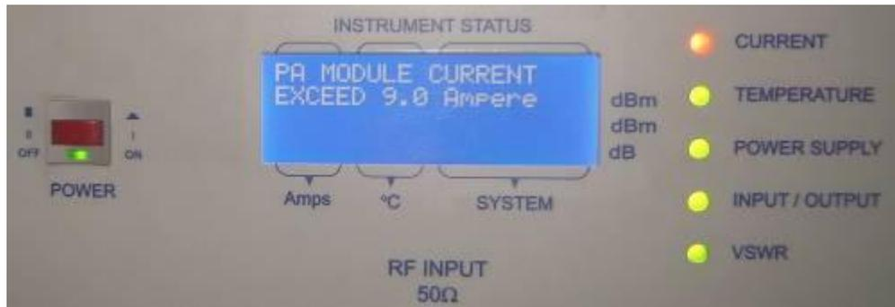
8. In order to restart the unit, first turn off the front panel switch, and then restart the unit as described in Section 3.
