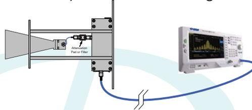
**FIGURE 9 - Typical setup for ACTIVE-Rx (non-std) mode**
