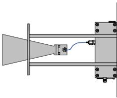
The provided *ACTIVE* Antenna Factors include all gain/loss factors for the assembly (pictured), up to and including the preamplifier output port connector. It includes the factor of the antenna, the insertion loss of the coaxial jumper cable and the preamplifier gain, calibrated as a system (not separately as individual components).
