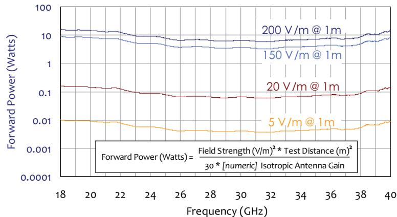
**FIGURE 15 - Power requirements for various fields strengths/distances**
