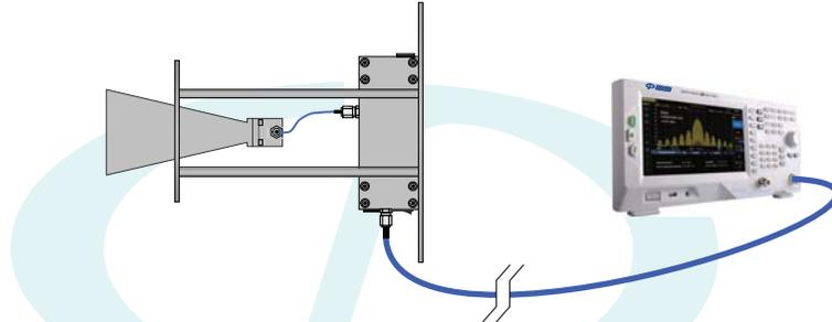
**FIGURE 7 - Typical setup for ACTIVE-Rx (Std) mode**
