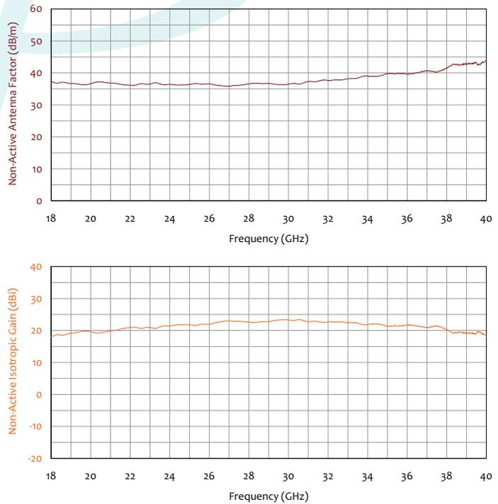
**FIGURE 17 - Typical NON-ACTIVE Antenna Factors/Gain Values**
