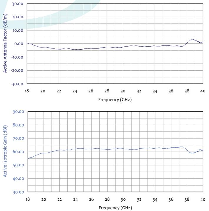
**FIGURE 16 - Typical ACTIVE Antenna Factors/Gain Values**
