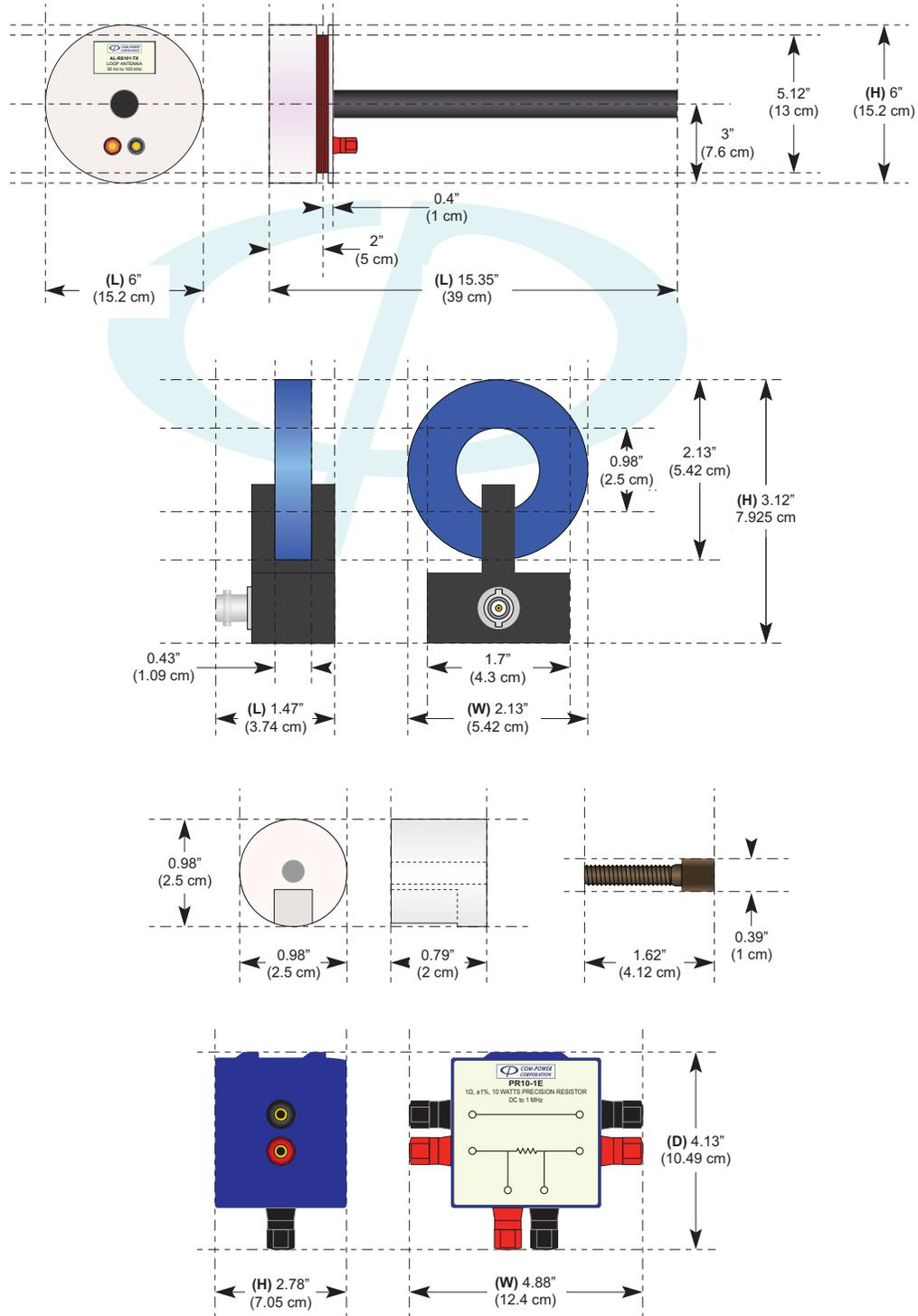
**FIGURE 3 - Dimensions of Loop Antennas and Accessories**
