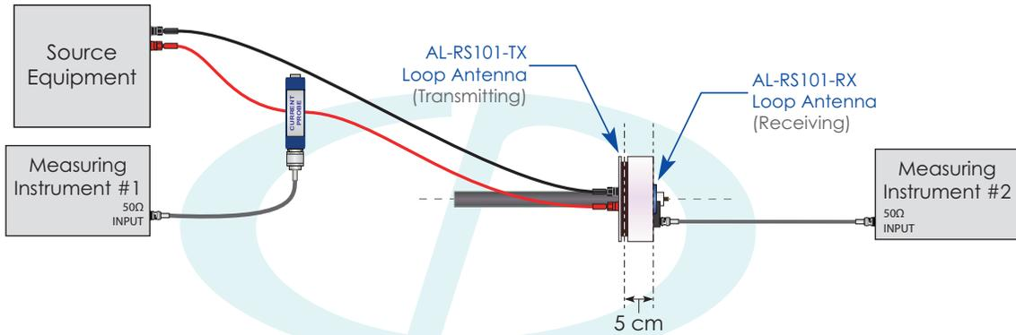
**FIGURE 5 - Setup Diagram for Test Level Calibration**
