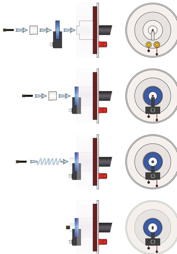
**FIGURE 4 - Mounting the AL-RS101-RX onto the AL-RS101-TX**
