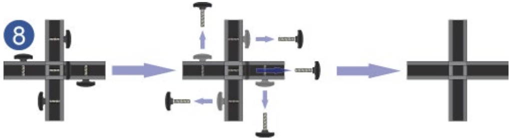
Figure 5 - ALT-930-2M Triple Loop Antenna Assembly – Step #1
