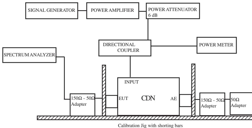
Figure 2-5 Level measurement setup using CDN
