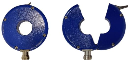
The current is measured inductively by clamping the probe around the line(s) to be tested. Essentially, a current probe is a toroidal transformer, with the line(s) under test acting as the primary, and the probe itself acting as the secondary. The probe's output voltage is measured across the 50Ω input impedance of the measuring instrument. This voltage is then converted to current by applying the probe's transfer impedance factor:
