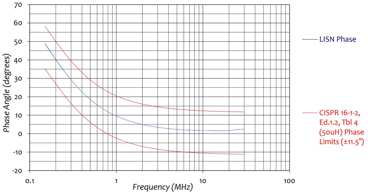
Figure 7: Typical Phase compared to CISPR 16-1-2 requirements.
