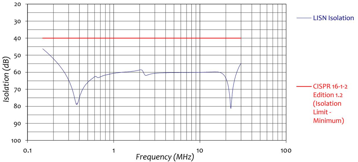
**Figure 8: Typical Isolation compared to CISPR 16-1-2 requirements**
