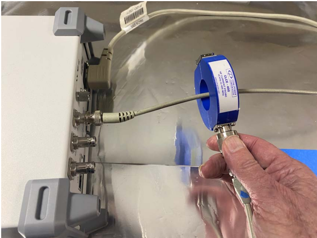
Figure 9 - Use of a current probe to measure high frequency currents flowing on I/O and power cables.
