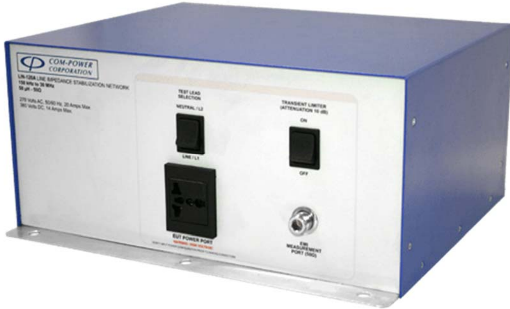
Figure 3 - An example of Com-Power's most popular LISN, the model LIN-120C.
