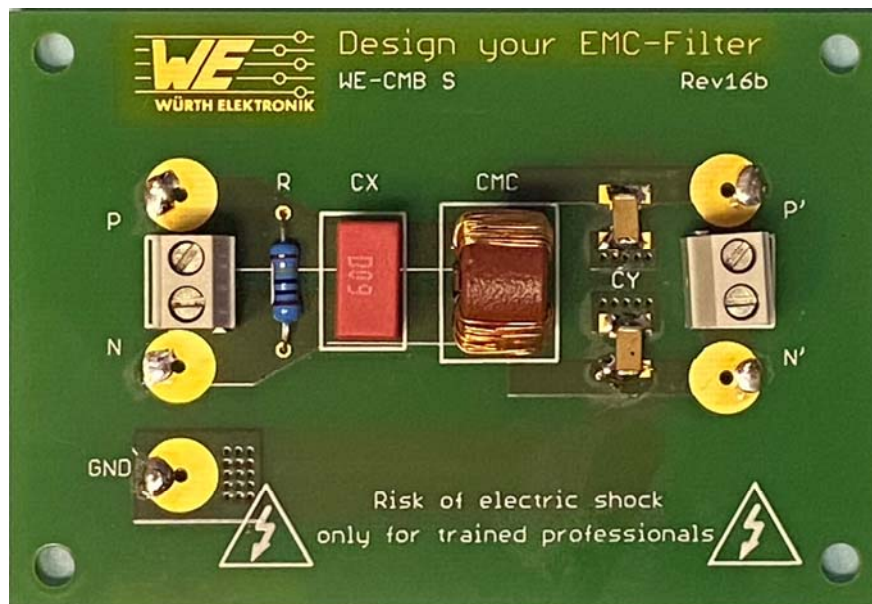
Figure 7 - This is the filter board from the Würth Elektronik filter kit with components added to suppress conducted emissions in the range 10 kHz to 30 MHz.
