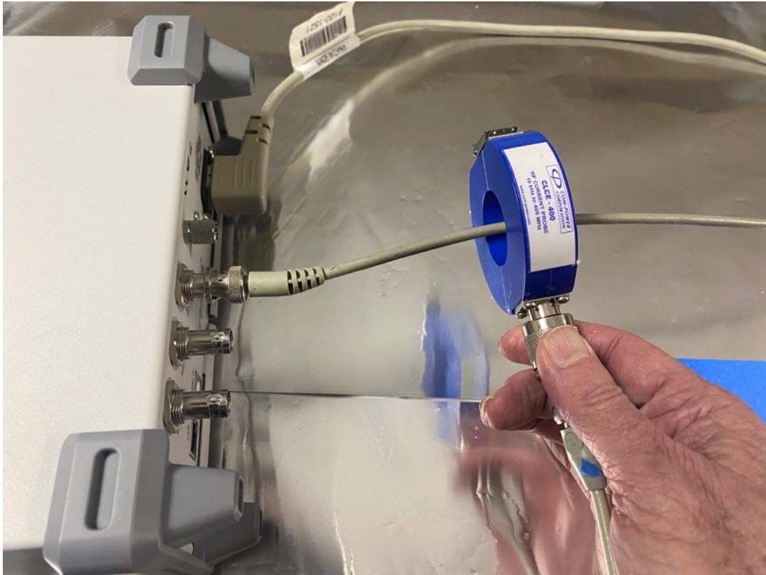
Figure 5 - Use of a current probe to measure high frequency currents flowing on I/O and power cables.
